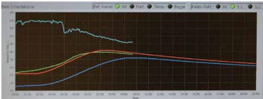
**Fig. 4:** Detailed view of a data plot. The dark blue line shows the initial predicted temperature history, the red line shows the temperature history of the last placement, the green line shows the actual temperature history, and the light blue line shows actual ambient relative humidity. As can be seen from the light blue line, the relative humidity dropped slightly about 4 hours into the curing cycle. This coincides with the opening of exterior doors, which briefly let in cold air
